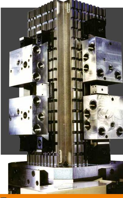
The components you wish to hold are clamped against a fixed jaw, and this jaw gives accurate location of each component in X, Y, and Z to aid programming.
